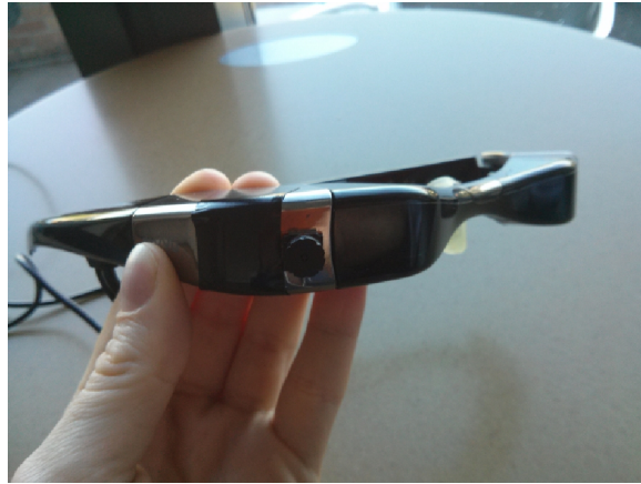
Figure 3.1: A photo of the mockup device worn during field sessions. The device is a Myvu Crystal Personal Media Viewer with an attached (non-functioning) camera.
